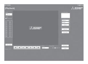
The function of searching for recorded picture data is effective only when the single-screen display has been selected in the "Playback" menu. The function cannot operate during picture data playback so to make a search of any type first stop the playback.
